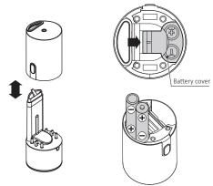
AAA alkaline batteries and AAA NiMH batteries can be used
